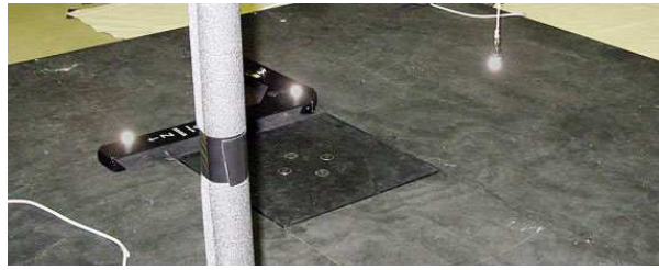
Figure 2.14: Photograph of load cell plate installed in motion capture platform.
